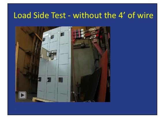
This test was conducted to verify the open door results of a load side fault. Fine-strand bare #10 SIS wire was connected in a short-circuit between the three load terminals.
