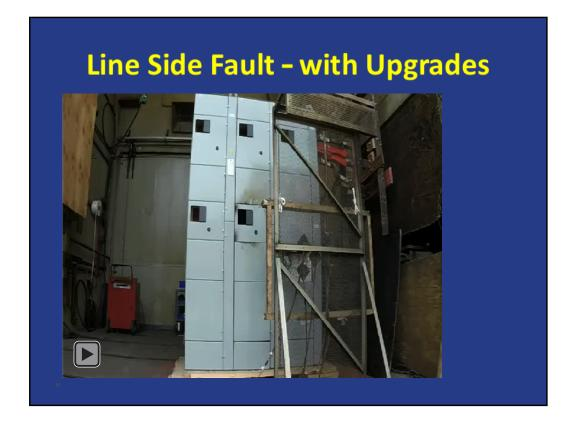
This is the combined result of the modifications in a Line Side fault. This is a 65kA fault, duration 9ms , the average calorimeter reading was .32 cal/cm<sub>2</sub>.
