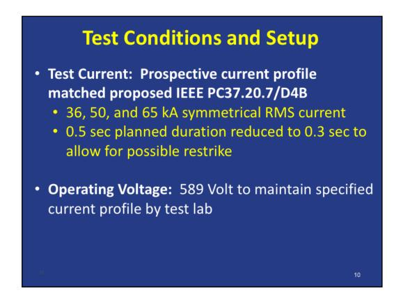
This was much worse than real life for a 480V system with the test voltage at 589V. As mentioned in Slide 8, the arc physics dictate that the duration where any free electrons are present is extremely short. Reducing the duration time actually makes the available energy the best case condition for arc restrike on this system configuration.
