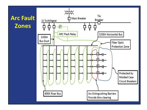
MCCB did show degradation for this close in fault but still performed well. This had to be confirmed since the UL testing requires the addition on the 4feet of rated wire to assure the feeder wire is protected by the components under test. In typical troubleshooting activities, the components are accessed at the terminals, creating the possibility of a close in fault condition.
