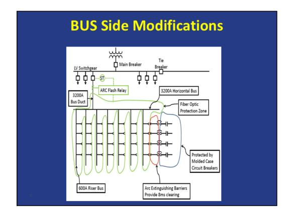
By adding the fiber optic sensors in the rear compartment, we were able to sense any light emitted by an arcing fault. By adding an Arc Flash Detection Relay (AFDR), current transformers on the feeder conductors, and a shunt trip device on the feeder breaker, we were able to create a separate static monitoring system independent of the existing time current coordination settings, yet trip extremely fast when both light and current are detected.
