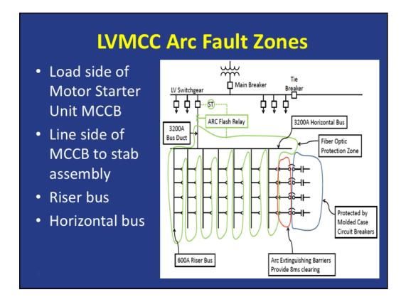
LVMCC is considered metal enclosed in design, meaning it does not have steel barriers between compartments or areas. In the simplest terms, it is one big box of components, wireways and busbars. It is true, however, that there is segregation between units and structures with a common rear area. Therefore we determined to look at the assembly on a "source of fault" basis. (i.e. where could a mistake or situation lead to a fault occurring?) That is what generated these areas –
