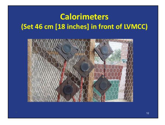
Purpose was to monitor the heat energy in calories. Mounted 18 inches from face of structure.
