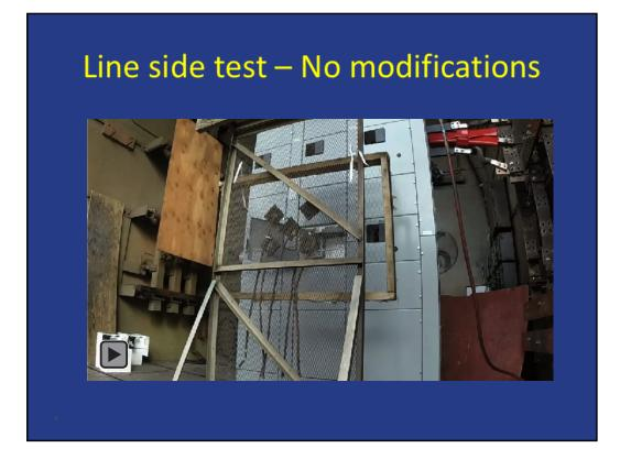
Five calorimeters placed at 18" from front of open door to measure heat energy from fault through open door. The configuration is bare #10 fine-strand SIS wire in a short circuit in the line side breaker terminals (see Slide 16), simulating a fault that could occur by a technician mistake measuring incoming voltage or expulsion of a lead wire during a load side fault. The fault current for this test was 50kA.
