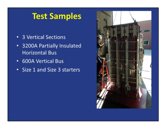
30A, 60A and 225A breakers were tested to verify ampacity was not a factor in the trials, which proved to be true.
