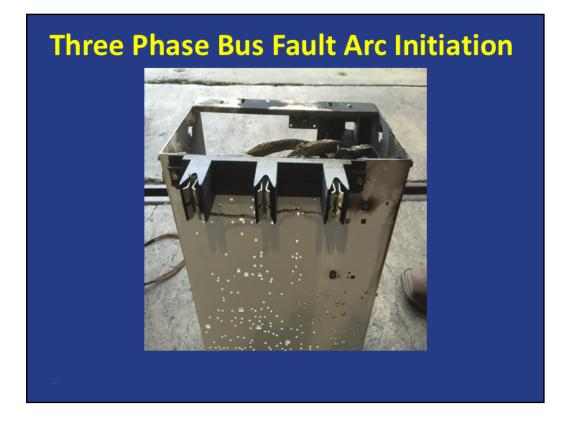
The #10 fine-strand bare SIS was installed by wrapping it through and around the stab assembly, creating a direct short circuit at the riser bus. This allowed the test plan to evaluate the arc flash relay application performance.
