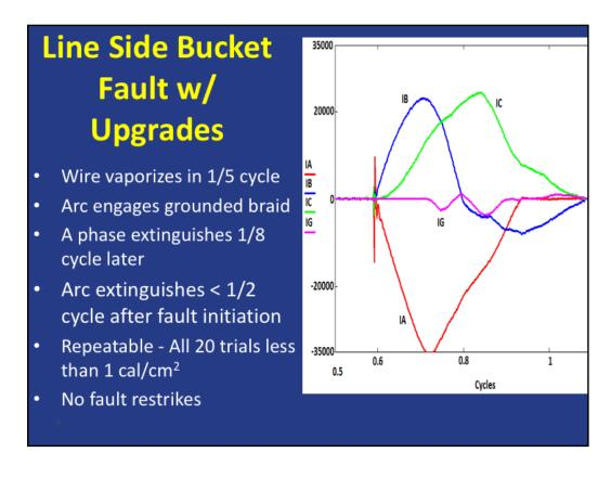
This profile was typical of all 20 tests after modifications were made to buckets.
