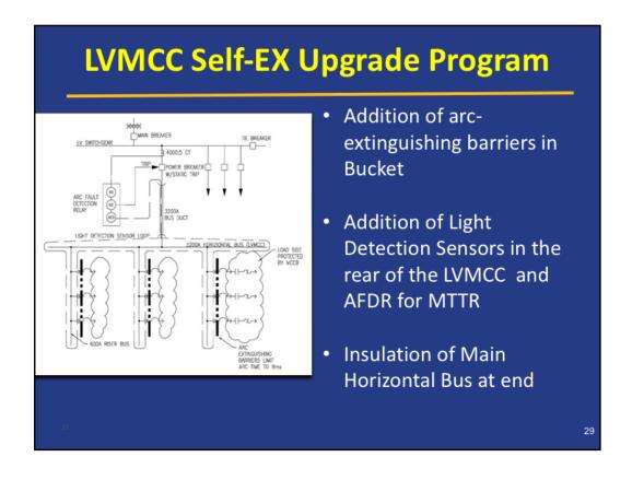
Another representation of the installed modifications and AFDR. The system only allows the AFDR to operate in the presence of both current and light – a true indication of equipment failure which would require service interruption. It was also proven that a fault within the bucket stays within the bucket and will not cause nuisance and dangerous interruption to critical plant processes by propagation to the rear compartment.
