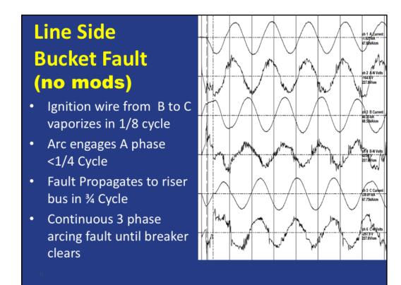
Waveform layout from top - A current, A-N Voltage, B current, B-N Voltage, C current, C-N Voltage Fault was initiated B-C phase, vaporized and initiated A phase within 1/8 cycle Propagates to rear bus in ¾ cycle where it continued until Main Backup Breaker de-energized circuit
