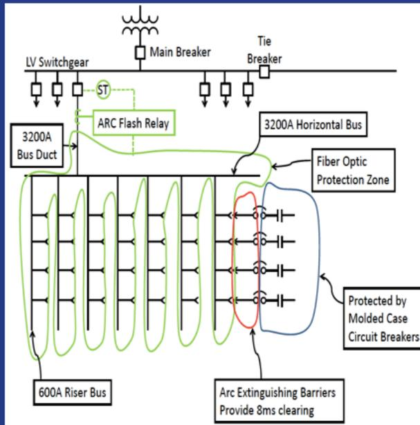
LVMCC is considered metal enclosed in design, meaning it does not have steel barriers between compartments or areas. In the simplest terms, it is one big box of components, wireways and busbars. It is true, however, that there is segregation between units and structures with a common rear area. Therefore we determined to look at the assembly on a “source of fault” basis. ( i.e. where could a mistake or situation lead to a fault occurring?) That is what generated these areas –
