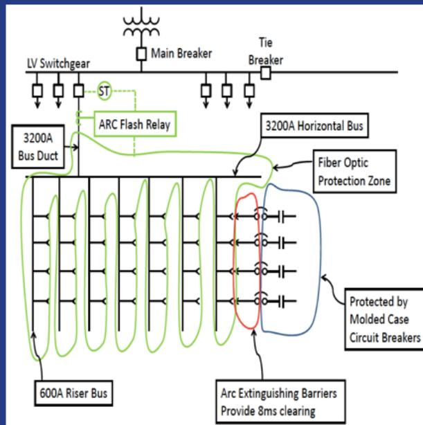
By adding the fiber optic sensors in the rear compartment, we were able to sense any light emitted by an arcing fault. By adding an Arc Flash Detection Relay (AFDR), current transformers on the feeder conductors, and a shunt trip device on the feeder breaker, we were able to create a separate static monitoring system independent of the existing time current coordination settings, yet trip extremely fast when both light and current are detected.
