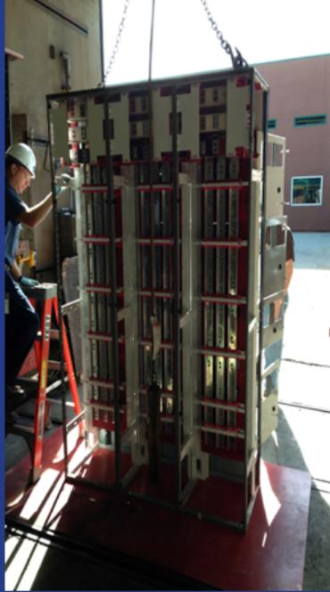
30A, 60A and 225A breakers were tested to verify ampacity was not a factor in the trials, which proved to be true.
